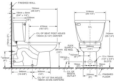
WASTE OUTLET SEAL RING MUST BE NEOPRENE OR GRAPHITE-
