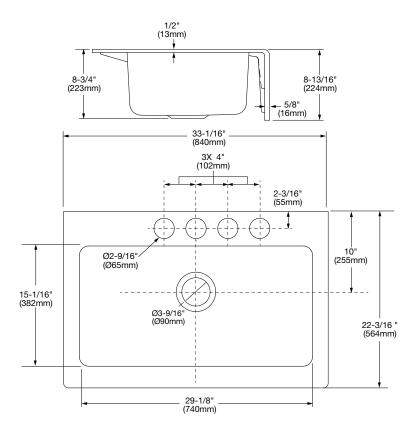
\*\* DIMENSIONS SHOWN FOR LOCATION OF SUPPLIES AND "P" TRAP ARE SUGGESTED. FITTINGS NOT INCLUDED WITH FIXTURE AND MUST BE ORDERED SEPARATELY. SEALING COMPOUND SUPPLIED BY OTHERS.
