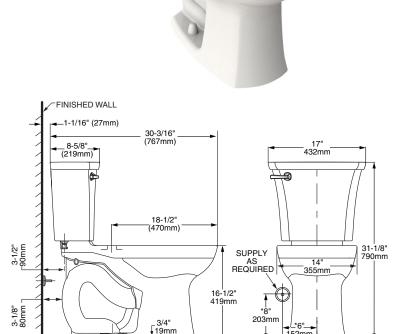
THIS TOILET IS DESIGNED TO ROUGH-IN AT A MINIMUM DIMENSION OF 305MM (12") FROM FINISHED WALL TO C/L OF OUTLET. SUPPLY NOT INCLUDED WITH FIXTURE AND MUST BE ORDERED SEPARATELY. \* DIMENSION SHOWN FOR LOCATION OF SUPPLY IS SUGGESTED.
